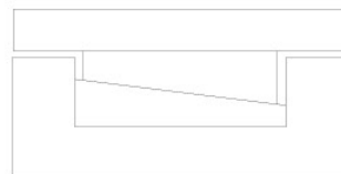
机械补偿剖视图 Sectional view of mechanical crowning compensation
